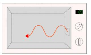
oven you should see a number in GHz (billion vibrations a second) or MHz (million vibrations a second), this is the number of waves the microwave produces every second - the frequency. Most microwaves produce electromagnetic waves with frequencies around 2.5 gigahertz – 2,500,000,000 Hz. Two billion, five hundred million vibrations every second.
